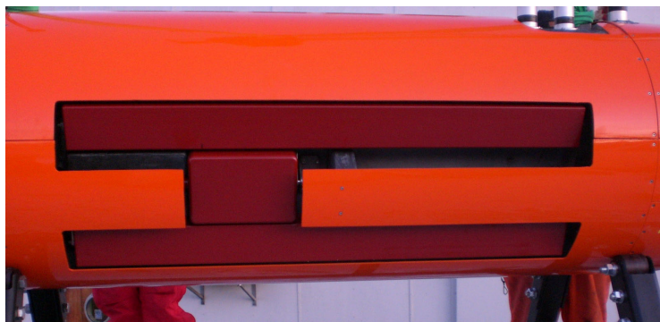
Figure 3: HISAS transducer arrays on HUGIN 1000-MR
