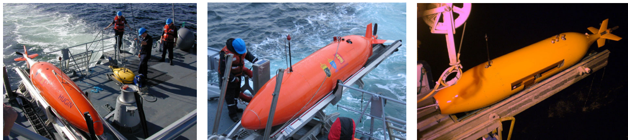
Figure 1: Three generations of RNoN AUVs. Left: The HUGIN I AUV onboard the RNoN MCM vessel HNoMS Karmoy , 2002. Centre: The HUGIN 1000 pilot system being launched from the same MCMV, 2004. Right: The HUGIN 1000-MR AUV being recovered after a sea trial, 2007.
